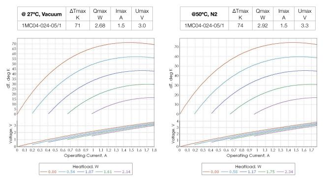
**Note**: Performance data is specified at optimal optimal conditions (TEC hot side is stabilized at ambient temperature). Any heatsink thermal resistance is not included into estimations. Use TECCad Software for estimations under different conditions.
